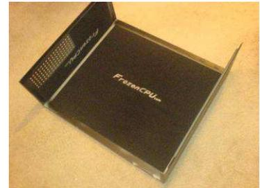
The LS13 ships with a front 92mm intake fan and twin 60mm exhaust fans at back. Most of the reviews found these fans to be somewhat less-than-quiet so they were removed, to be replaced by other fans that have been well-tested as to be virtually silent.
