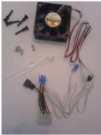
To bring the sound down further, it is under-volted to 7V by using a Zalman 56-ohm in-line resistor, a device similar to the Noctua LNA. At 7V the fan is probably running at about half CFM & RPM. All this under-volting might seem a little nervy. But, again, it can be changed out very quickly, need be. And besides the generous ventilation provided by the Seasonic, there's plans for a bit more compensating air yet to come. The AcoustiFans arrived
