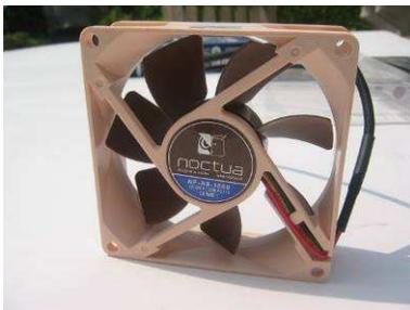
At 12V, the Noctua runs 31CFM, 1800RPM, 17dBA (Less than 19 dBA is considered inaudible). This is highest CFM/dBA ratio on the market. I also used the supplied “LNA”—Low Noise
